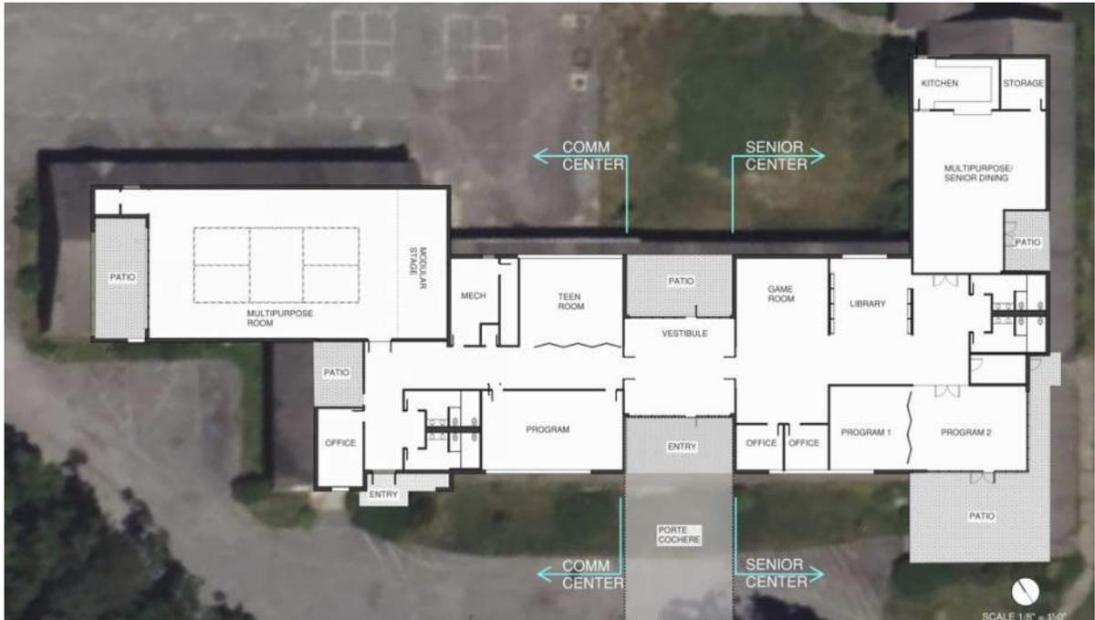
*Figure 15: Development Option 2 – Floor Plan*
